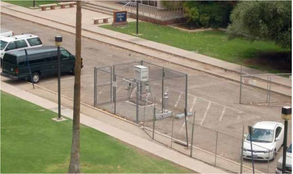
Figure 1. U.S. Historical Climatology Network weather station used to collect climate data. This station is located in a parking lot at the University of Arizona in Tucson. The station was previously located in a grassy area, but researchers moved the station as the campus grew. Photo by Anthony Watts.
